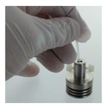
Locate the tip of the stent into the LGC
