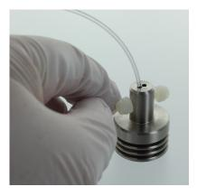
Lightly tighten the nylon screws to secure the stent DO NOT OVERTIGHTEN
