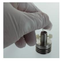
Gently insert the stent 12-15mm until it reaches the bottom of the LGC barrel
